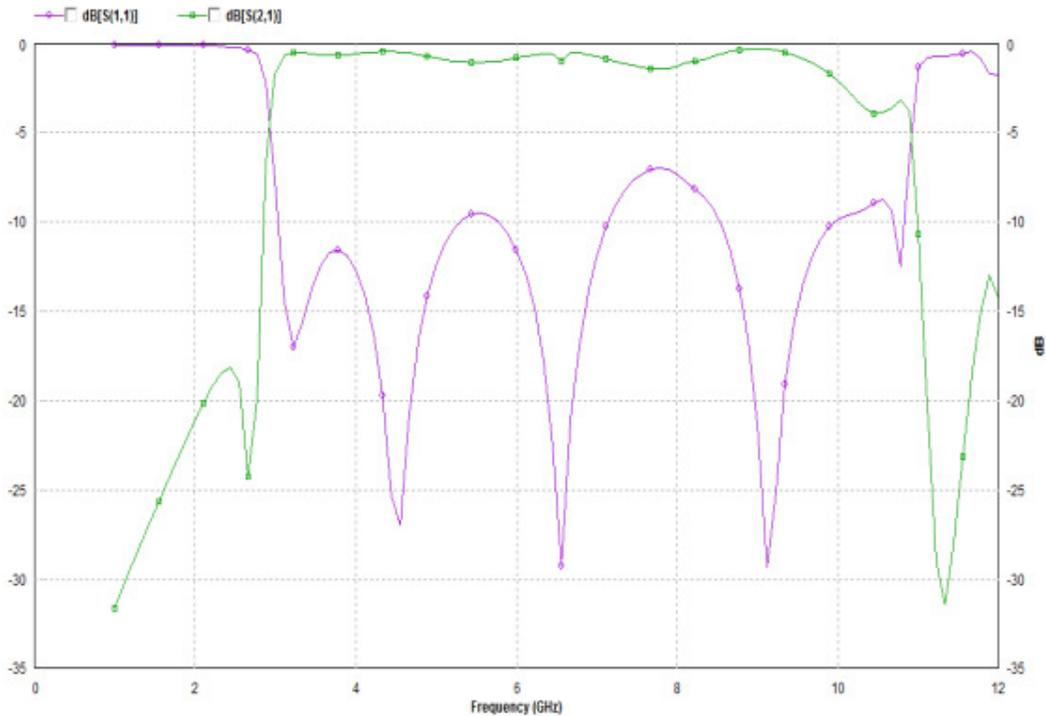
**Fig.8 Simulation Results of Stepped Impedance Stub Loaded Resonator**
