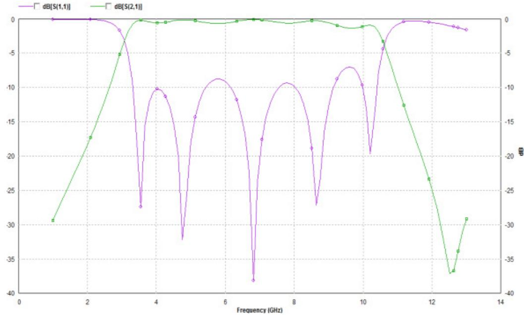
**Fig.9 Simulation Results of Multiple Mode Resonators**
