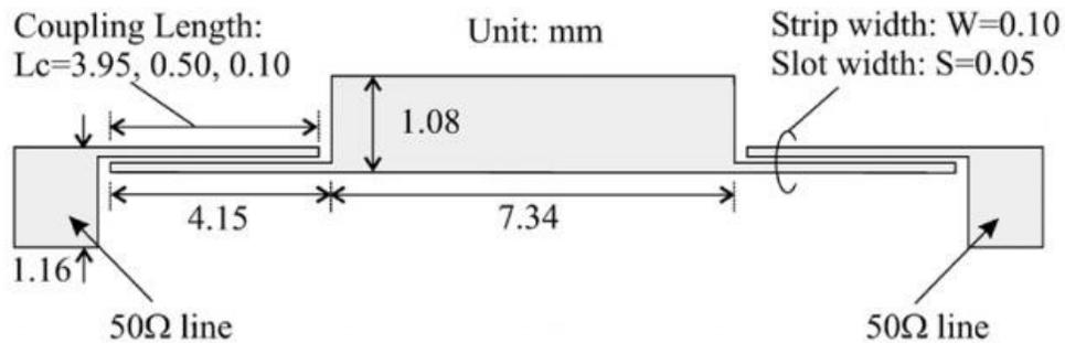
**Fig.6 Basic Multiple-Mode Resonator**
