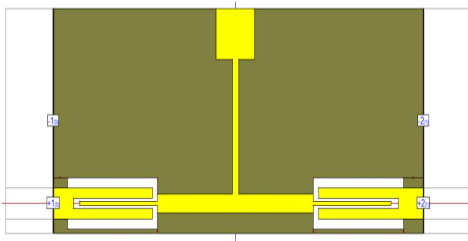
**Fig.5 Stepped Impedance Stub Loaded Resonator.**
