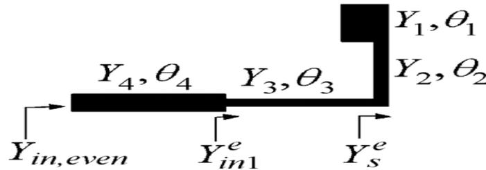
Fig 4: Basic structure of SISLR, even-mode equivalent circuit.
