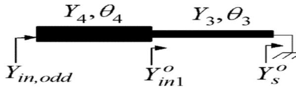
Fig.3 Basic structure SISLR, odd-mode equivalent circuit
