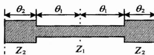
Fig.2 Basic Structure of SIR (Half Wavelength type)
