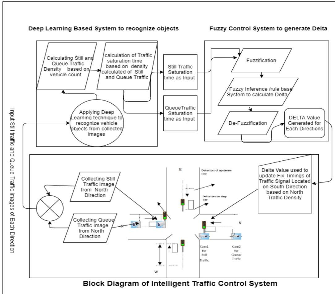
Figure.6. Block Diagram of proposed designed intelligent traffic control system
