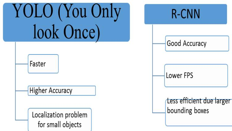
Figure. 4 Comparison of Object detection methods
