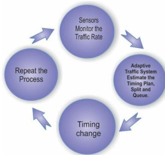
**Figure. 2. Working of Adaptive Traffic Signal Control [2]**
