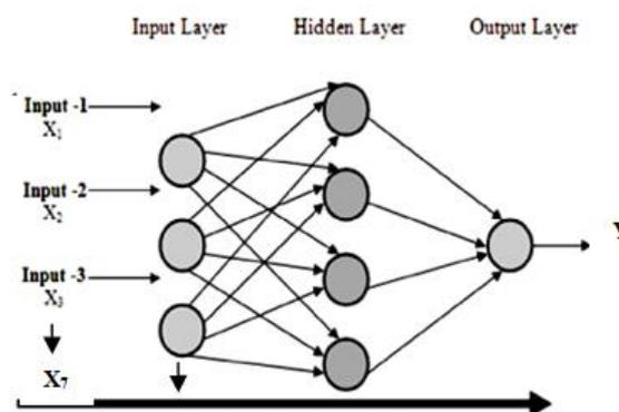
Here is the procedure given to fix the number of hidden layers. Majority of problems need only one hidden layer, since it is better those NNs with more hidden layers are extremely hard to train. The following method can be used in setting the hidden layer configuration using the following rules:
