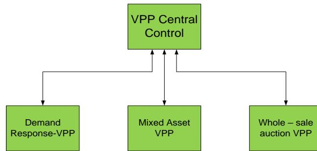
Fig. 4: Domain specific segmentation of virtual power plant
