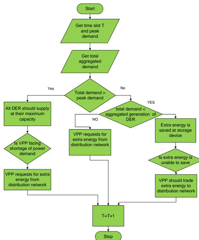
Fig. 2: Flow chart, how VPP deals with aggregated demand and aggregated generation
