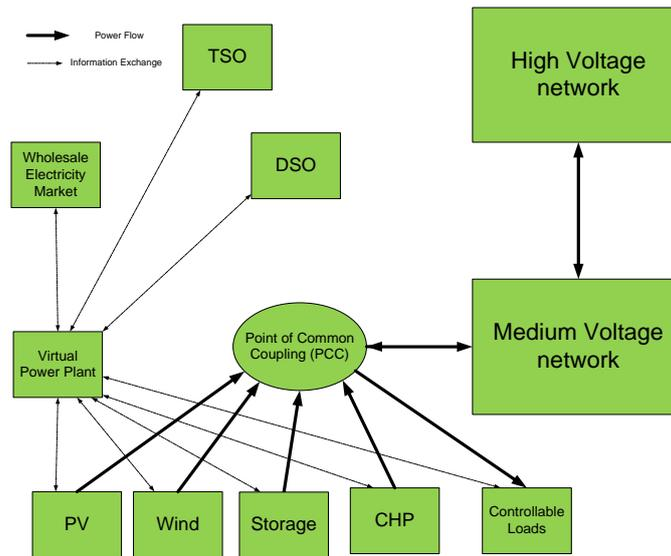
Fig. 1: Basic Architecture of Virtual Power Plant
