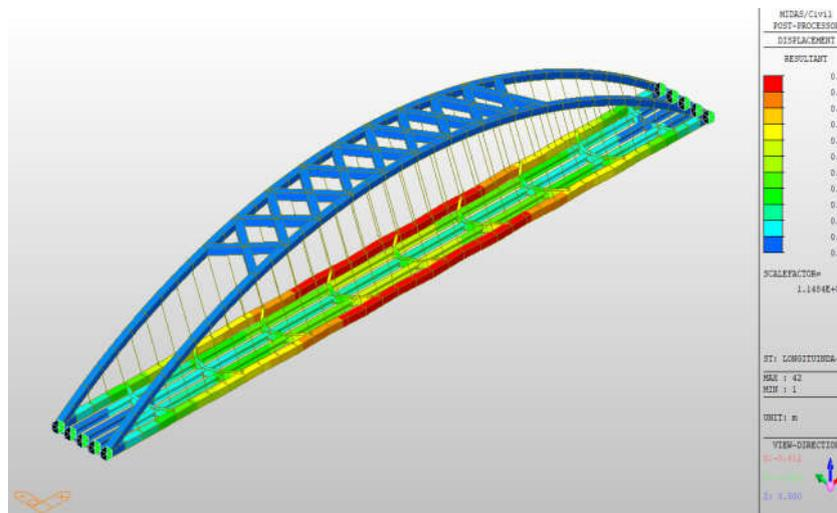
Figure 10. Deformation due Longitudinal Wind Force
