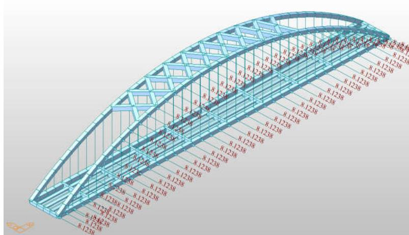
Figure 6. Transverse Wind Load on Single Tied Arch Bridge.
