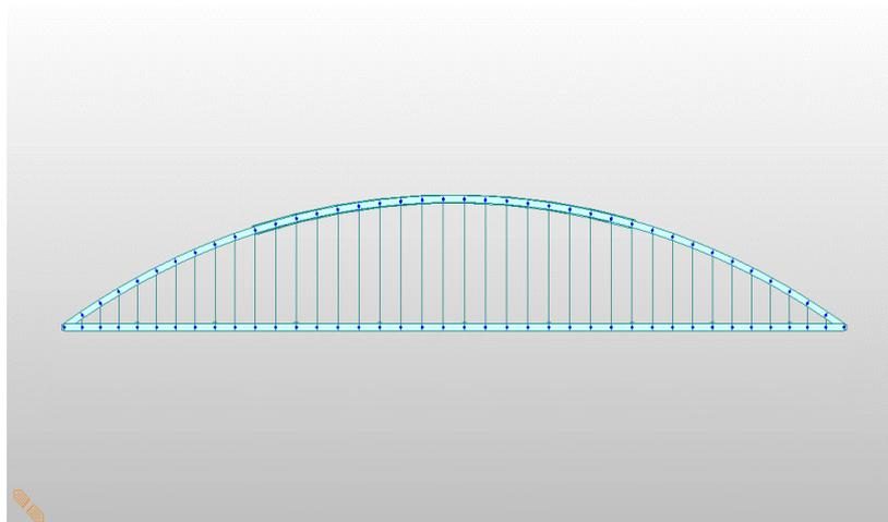
**Figure 4 Section View of Single Tied Arch Bridge.**
