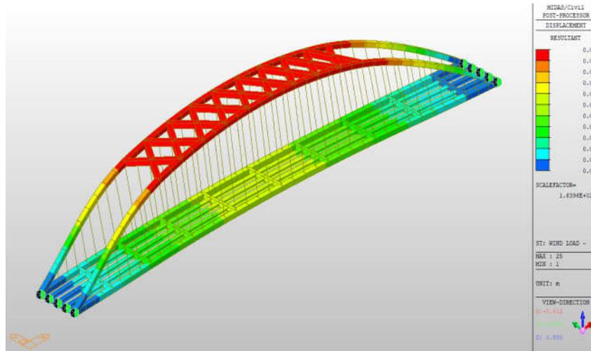
Figure 9. Deformations due to Transverse wind load
