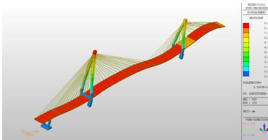
Figure 7. Deformation due Longitudinal Wind Force
