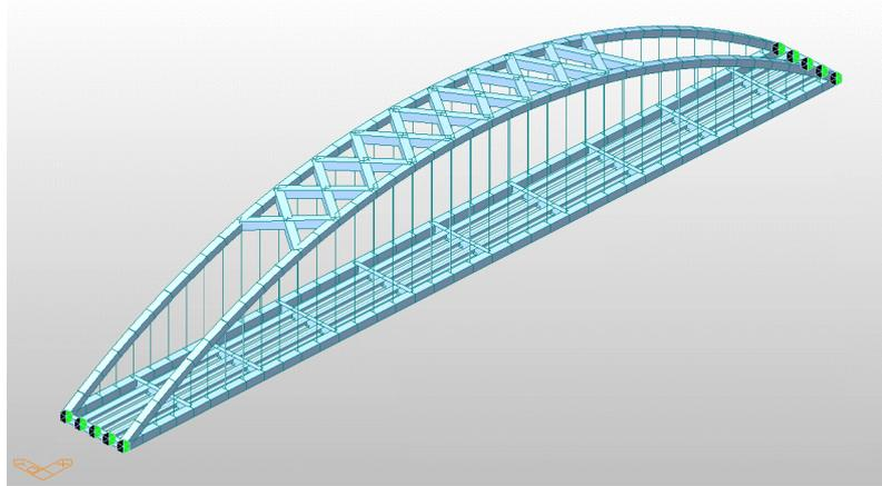
Figure 5. Supports of Single Tied Arch Bridge.
