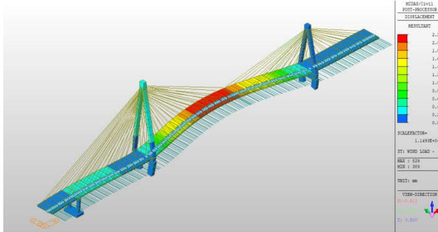
Figure 8. Deformation due to Transverse wind load
