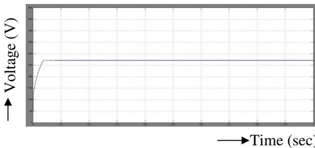
Figure 15. Output voltage waveform of Modified SEPIC converter with coupling in closed loop configuration
