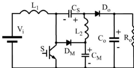
Figure 1. Modified SEPIC converter without coupling
