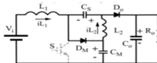
Figure 2. Modified SEPIC without when switch is turned off
