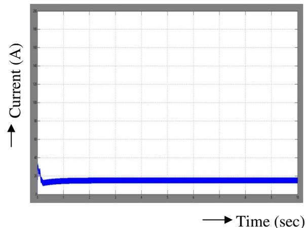
Figure 9. Input current waveform of Modified SEPIC converter without coupling in closed loop configuration
