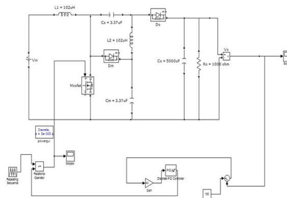
Figure 6. Modified SEPIC converter without coupling in closed loop configuration
