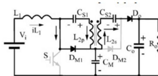
Figure 4. Modified SEPIC converter with coupling and a voltage multiplier cell
