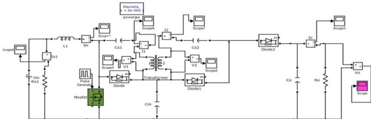
Figure 12. Modified SEPIC converter with coupling in open loop configuration
