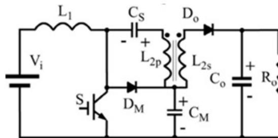
Figure 3. Modified SEPIC without coupling when switch is turned on
