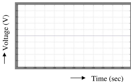
Figure 7. Input voltage waveform of Modified SEPIC converter without coupling in closed loop configuration
