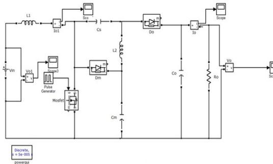
Figure 5. Modified SEPIC converter without coupling in open loop configuration
