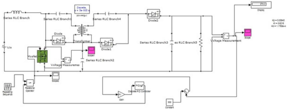
Figure 13. Modified SEPIC converter with coupling in closed loop configuration
