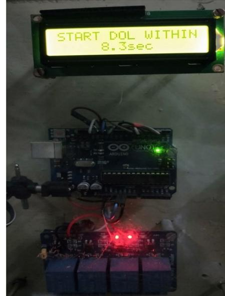
Fig. 3. LCD showing countdown to start DOL
