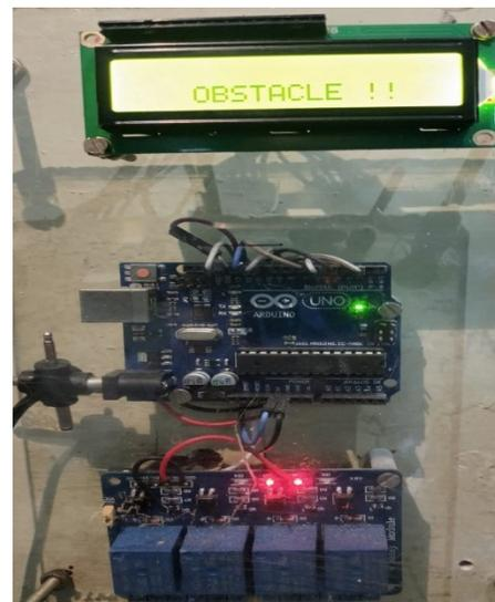
Fig. 4. LCD showing sensing status
