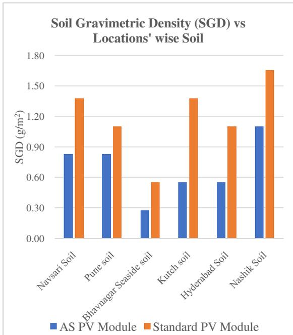
Fig. 6 Soil Gravimetric Density (SGD) of AS and Standard PV Module for Different Locations' soil
