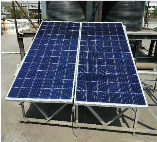
Fig.2 Anti-soiling (AS) PV Module (Left) and Standard PV Module (Right)
