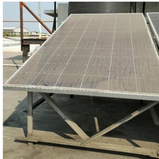
Fig. 1 Soiled PV Module
