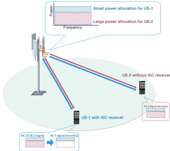
Figure 1: Non-Orthogonal Multiple Access
